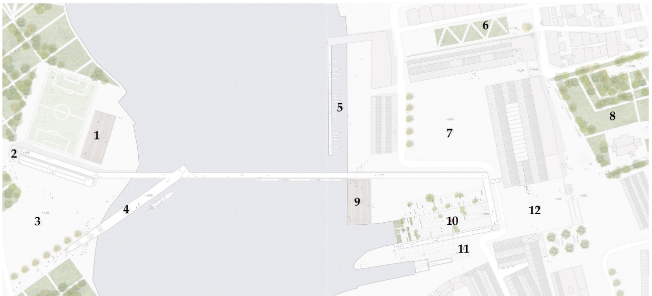
Fig. 6. General plan of the pedestrian bridge and of the open public spaces it defines: 1) Sport Area; 2) Connection Tower to the bridge; 3) Park Square; 4) Vapur Dock; 5) Marina; 6) Underground Parking; 7) Events Square; 8) Aynalikavak Park; 9) Water Square; 10) Boat Ramp; 11) Market Area; 12) Museum Square.
